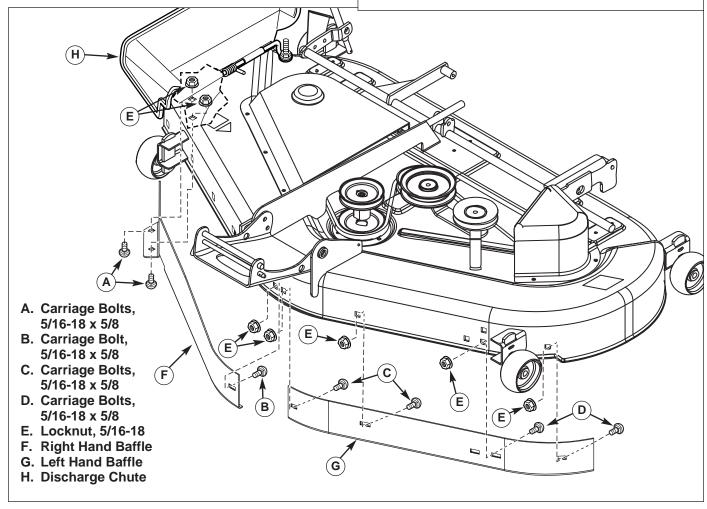
Figure 4. Baffle Assembly
